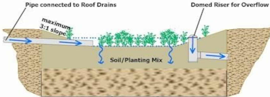
Figure 4: Cross-Section of Typical Rain Garden/Bioretention Area
